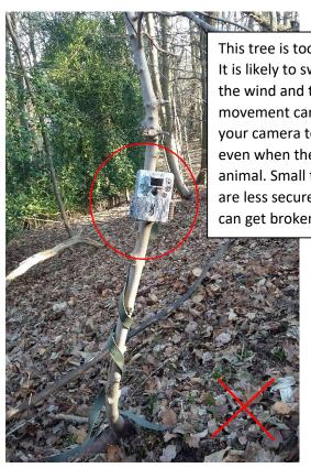
This tree is too small. It is likely to sway in the wind and this movement can cause your camera to trigger even when there is no animal. Small trees are less secure and can get broken.
