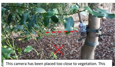
This camera has been placed too close to vegetation. This will obstruct the view of the camera and waving branches in the wind will cause false triggers (i.e. it will end up with lots of pictures of the bush and not much else!)
